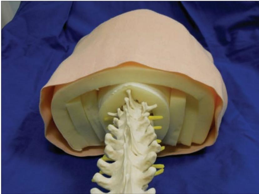
**Figure 1.** Photograph of the model showing the layers of coarse cellular foam and a flax cover around a commercially available spine model.
